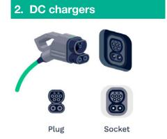
These chargers use additional ports to support three-phase or rapid DC charges known as CCS (Combined Charging System).
