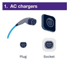
Australia uses Type 2 plug (for vehicles manufactured and sold after 2018). This is the plug used for all current vehicles imported into Australia. Type 2 is the standard plug compatible with AC chargers.
